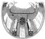
Looking aft toward tail cone of dehhwilled Homet. Seen are plywood skin and bulkheads and in foreground combination wood metal center back reinforcement.
